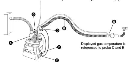
The humidification system is now set up and ready for use. After power on, the humidifier will operate in the last mode setting. Ensure that invasive mode is set for patients that have bypassed airways. Ensure that the humidifier is securely mounted.
