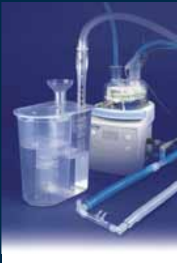
Infant Bubble CPAP therapy system, incorporating heated humidifier and water bubbling mechanism to create oscillating air pressure in the lungs
