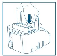
2. Push the filter grip firmly onto the low-pressure oxygen inlet port.
