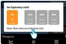
Select the level of expiratory relief desired. The flow rate is automatically reduced by the level selected as you exhale. When Off is selected, the flow rate doesn't change as you breath.
