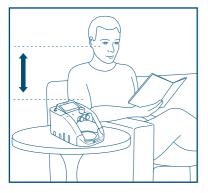
Before starting your therapy, you will need to ensure that the device is level and that the top of the humidifier is below head-height during therapy.
