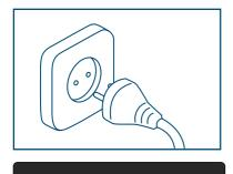
Plug the myAirvo 3 power cord into a power outlet. Position the myAirvo 3 so that the power cord connection to the wall power supply is easily accessible and can be disconnected if necessary.
