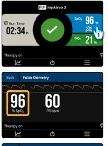
If SpO<sub>2</sub> value is displayed on the home screen, you can tap the pulse oximeter tile to open the Pulse Oximetry screen and view the pulse oximeter status.
