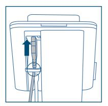
Plug the USB connector cable into either of the USB ports on the back of the myAirvo 3. Clip the pulse oximeter's cable into the cable tidy so that it is not pulled out accidentally. The myAirvo 3 will automatically detect a compatible pulse oximeter.
