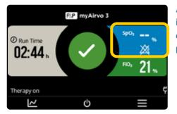
A '--' indicates that the pulse oximeter has been detected and is currently not returning a valid  $SpO_2$  value. Place the sensor on the measurement site and wait for the  $SpO_2$  value to populate.
