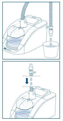
• Lowering the patient-interface end of the tube into a container. Place the container below the myAirvo 3 so that condensate runs into the container.
