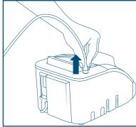
If you have been prescribed supplementary oxygen, connect your oxygen supply while the myAirvo 3 is warming up. Connect the tube from your oxygen supply to the oxygen port on the top of the myAirvo 3. Push the oxygen tube firmly onto the connector.
