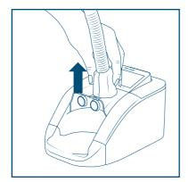
3. Detach the AirSpiral Tube from your myAirvo 3 by squeezing the sides of the AirSpiral Tube connector and pulling up. Drain any excess water from the AirSpiral Tube.
