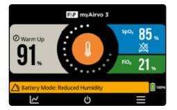
A battery may be fitted to your myAirvo 3 to prevent interruptions to your therapy during power outage. A battery symbol will be displayed in the Message bar if a battery is fitted.
