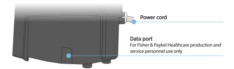
Caution: Do not remove data port cover during normal use. Removing the data port cover could cause the device to be vulnerable to malicious actions, or unintentional misuse, potentially increasing risk of patient harm.
