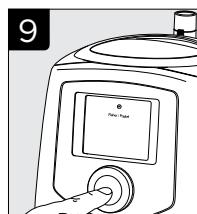
From the Home Screen, a quick press to the SmartDial™ will start therapy. The Home Screen will light up and the clock-face of the Menu System will rotate to indicate therapy is starting. If Ramp is required, press the SmartDial again and hold for 3 seconds to activate. The Ramp symbol ▾ will display.
