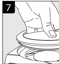
The Chamber Lid can be unlocked by twisting in an anti-clockwise direction, then removed by lifting away from the device.
