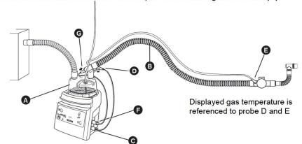
The humidification system is now set up and ready for use. After power on, the humidifier will operate in the last mode setting. Ensure that invasive mode is set for patients that have bypassed airways. Ensure that the humidifier is securely mounted.
