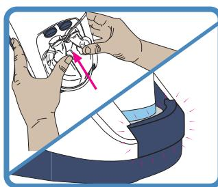
Fit the water chamber to the unit by pressing down the finger guard and sliding the chamber on, carefully aligning with the blue chamber port ends.
