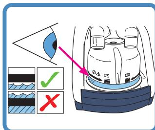
Check that water flows into the chamber and is maintained below the maximum water level line. If the water level rises above the maximum water level line, replace the chamber immediately.
