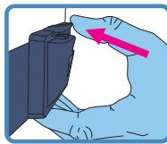
1. Take the filter holder from the back of the unit and remove the filter.
