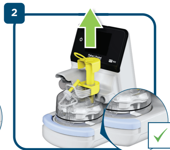
2 Pull ring to remove the yellow float retainer from the humidification chamber. Recycle or dispose of this yellow part.
