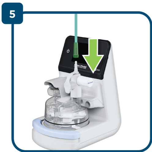
Connect the gas supply line to the BCPAP pressure relief manifold.
