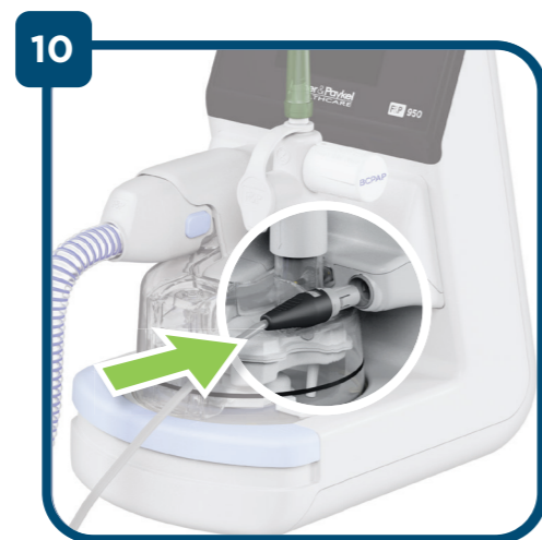
Connect the expiratory heaterwire adapter to the sensor cartridge.
