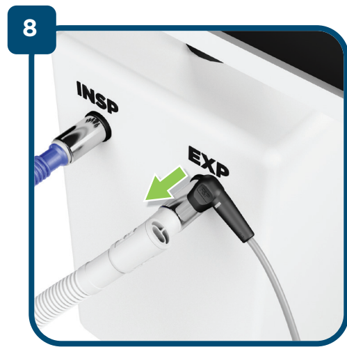
Connect the expiratory heater wire adapter to the expiratory limb.
