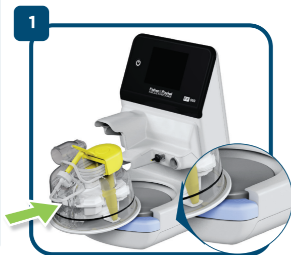
1 Press down on the blue finger guard and insert the humidification set.
