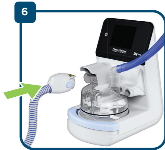
Connect the inspiratory limb to the humidification chamber.
