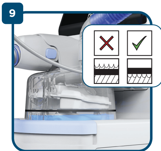
Ensure the water level in the humidification chamber is below the maximum line.
